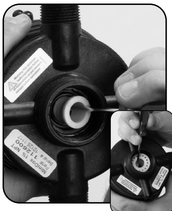
Step 7. Replace #82 SHAFT SEAL SPACER and #16 Gasket.
