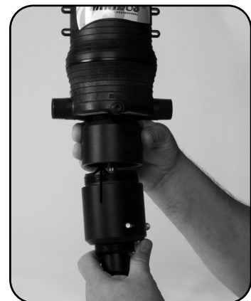
Step 9. Screw #61 OUTER CYLINDER onto body.
