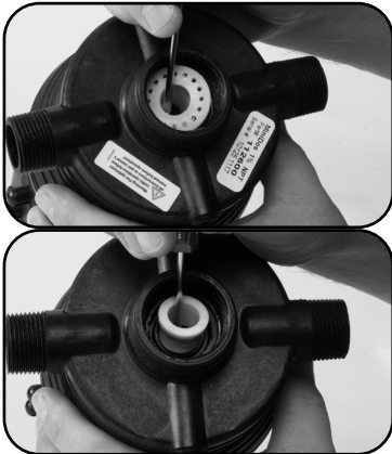
Step 4. Remove and clean #16 GASKET and # 82 SEAL SPACER.
