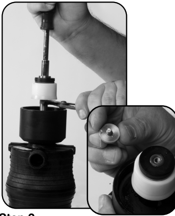
Step 2. Unscrew to unlock and remove #93 CAPSCREW.
