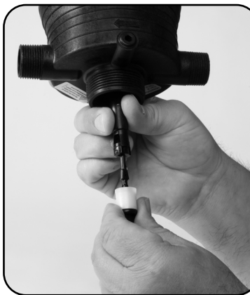
Step 8. Reinstall lower shaft with new dosage piston by turning 90° to lock in place.
