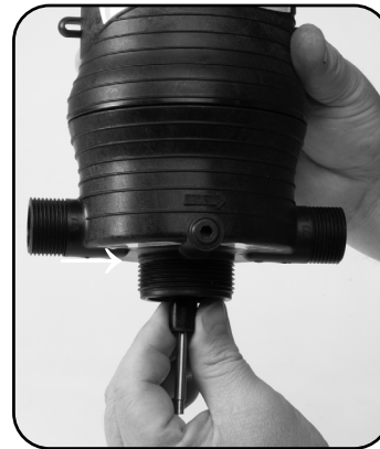
Step 6. After replacing #82 SEAL SPACER and #18 GASKET, replace #52 UPPER SHAFT. Turn 1/4 turn to lock in place.
