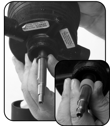
Step 6. Remove and replace #17 O-ring. Re-install #83 SHAFT SEAL SPACER and #15 SEAL RETAINER.
