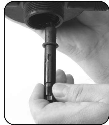
Step 6. Re-install #52 UPPER SHAFT and #17 O-ring.
