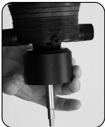
Step 7. Reset #68 O-ring and screw #72 ADAPTER onto body.
