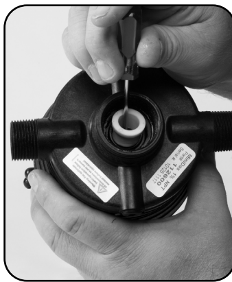
Step 5. Replace #83 SHAFT SEAL SPACER.
