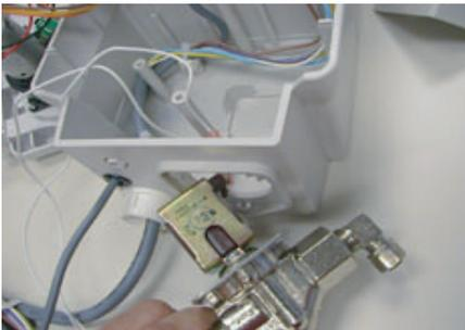
7. Feed solenoid wire harness through the opening in the bottom and tilt solenoid into place.
