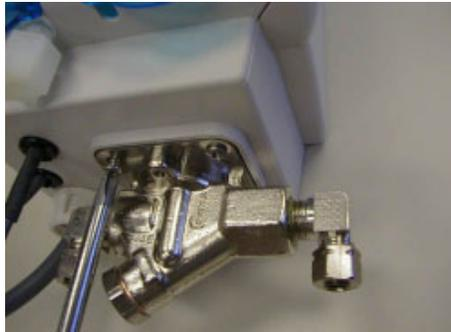
5. Replace the three thread-forming screws to hold bracketed solenoid in place.
