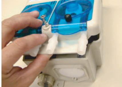
2. Open unit by lifting pump housing away from the unit
