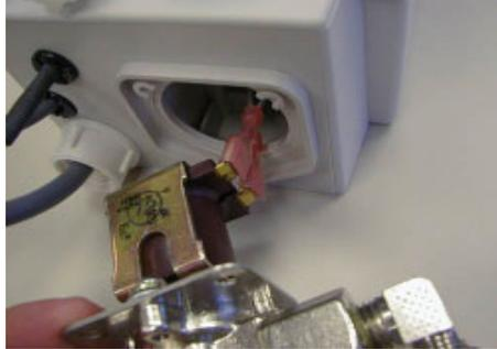
2. Tilt the solenoid as it is removed from the cabinet to allow the coil to clear.
