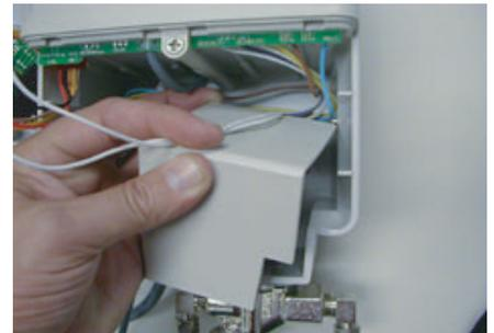
9. Guide solenoid wire harness through the notch in solenoid cover provided. Place cover over center boss and insure that it seats down to the back wall of unit.
