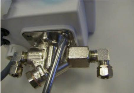
1. Remove the three screws that hold the bracketed solenoid in place.
