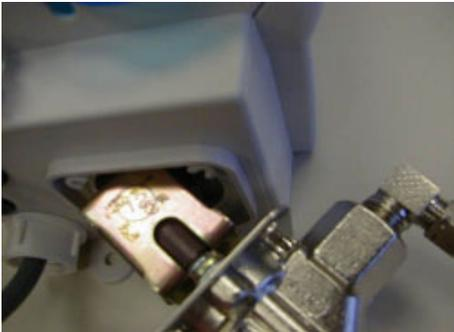
4. Tilt solenoid to insert coil making sure orientation is correct.
