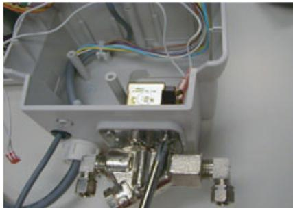
8. Attach solenoid to housing using the three thread-forming screws provided. Insure that screws are tight and solenoid is firmly in place.
