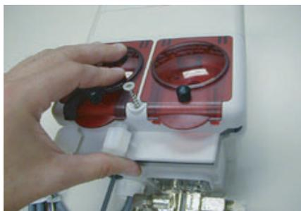
11. Replace pump housing. Make certain no wires are pinched between housings, tighten screw to secure
