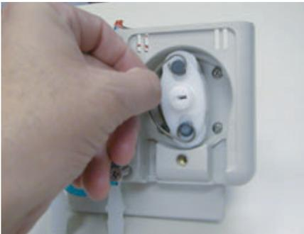
4. With pump housing removed, remove pump tubing and spinner assembly from the #2 position.
