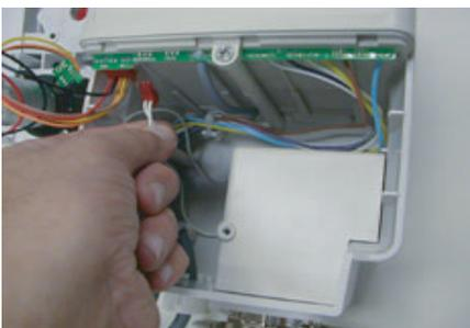
10. Make the connections for both the motor and solenoid
