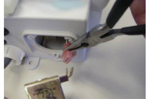
3. Remove (from old) and replace (onto new) the two QDC connections.
